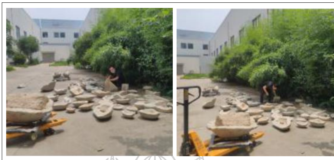
Figure 126 Drying (the finished mold contains a lot of moisture, which can be used after drying) (Photographed by Wang Yurong 2020)
