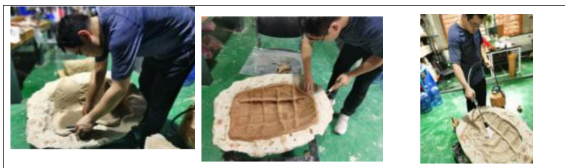
Figure 128 Make the mud piece fit the mold perfectly, and make a support to prevent the mud piece from collapsing (Photographed by Wang Yurong 2020)
