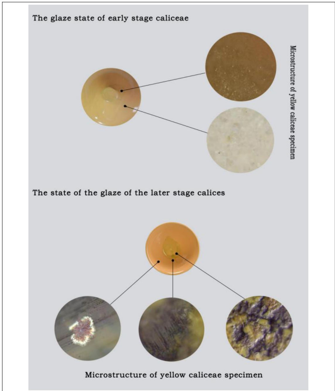
Figure 78 Microstructure of yellow caliceae specimen (Photographed by Feng Shanxin 2018)
