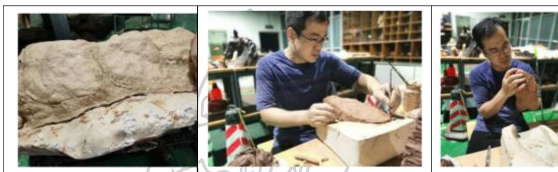
Figure 130 Taking out the body and repairing the mold line and details (Photographed by Wang Yurong 2020)
