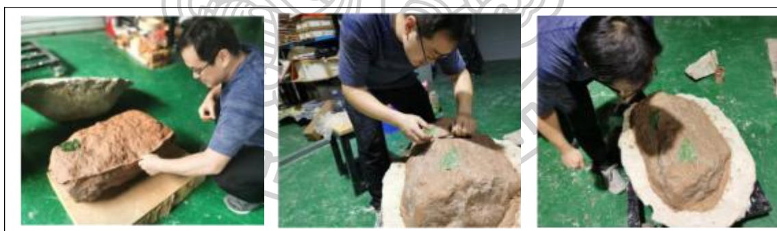
Figure 131 After the mold is turned over, the body is dried and put into the kiln for the first firing before the leaf is put in for glaze firing (Photographed by Wang Yurong 2020)
