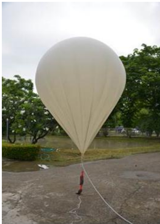
Figure 7.6 The balloon lifts Pendulum weight of 2 kg.
