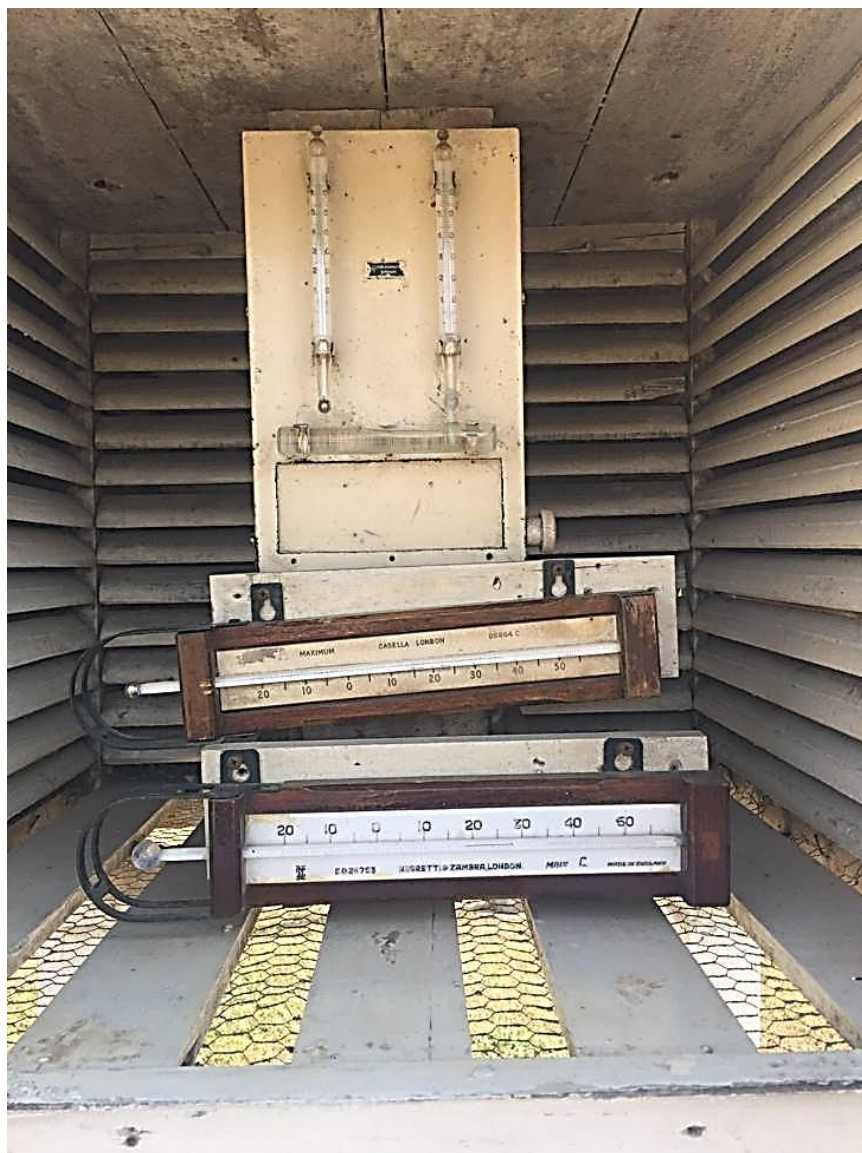
Figure 3.2 Psychrometer completed with wet-dry thermometers of the Thai Meteorological Department at Bangna, Bangkok.
