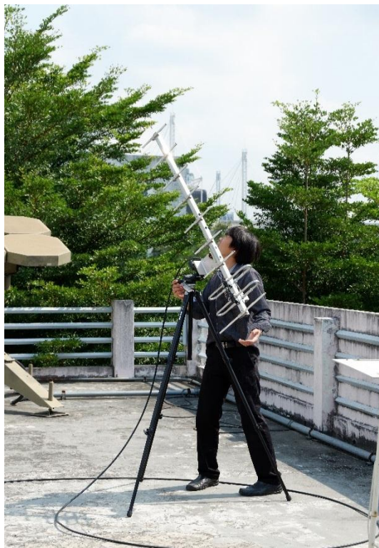
Figure 7.10 Antenna adjustment receive radio signals from the radiosonde.
