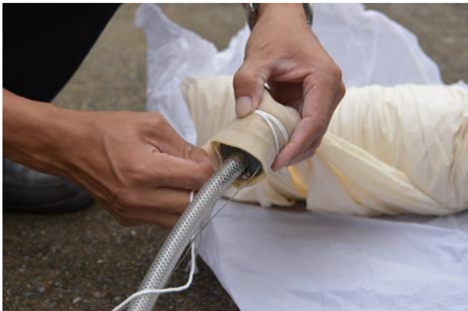
Figure 7.4 Attaching a balloon to a helium pipe.
