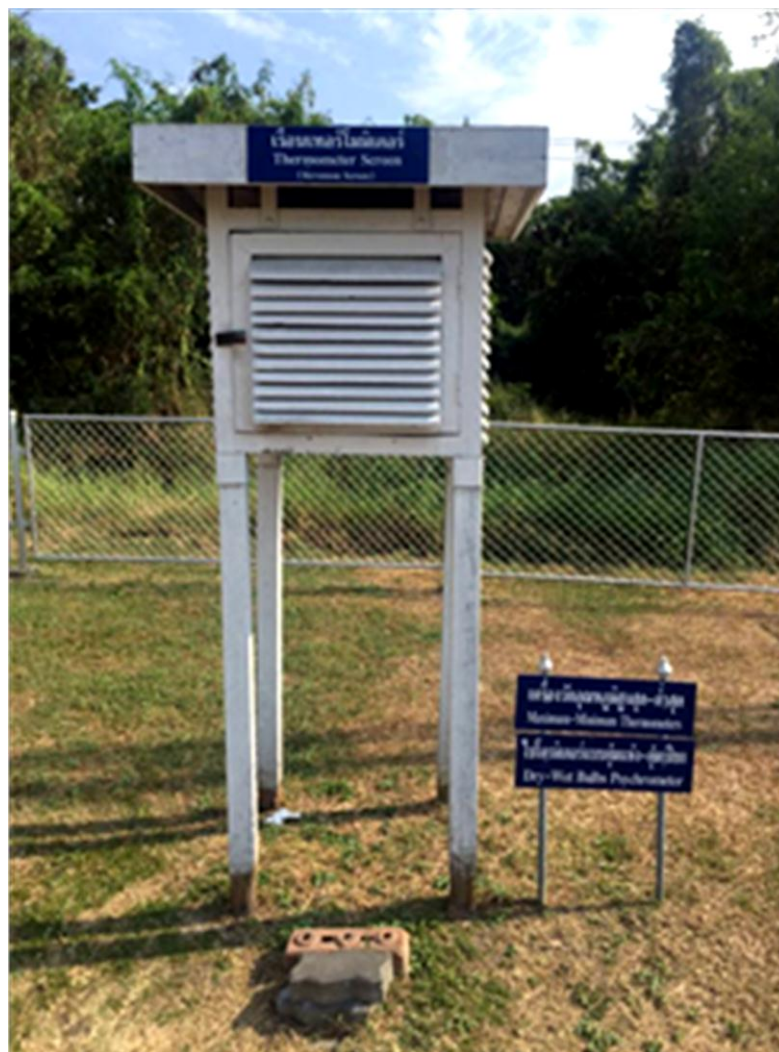
Figure 3.1 Thermometer screen cabinet of the Thai Meteorological Department at Bangna, Bangkok (TMD).
