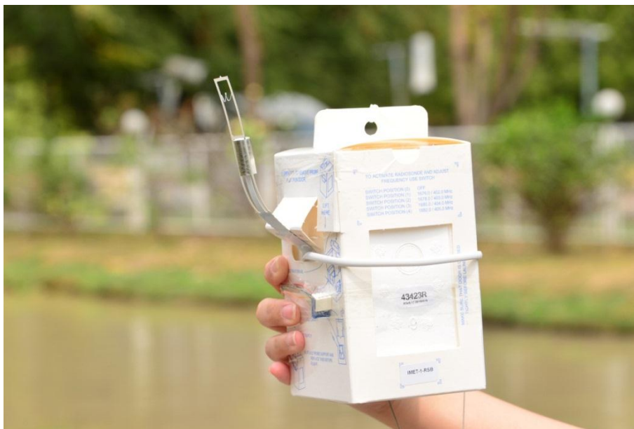
Figure 7.2 Internet iMet-1 radiosonde with temperature and humidity sensors.
