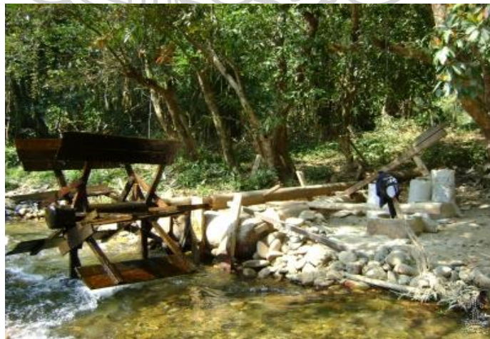
Figure 97: 'Sai Nam Tum Khaw' is a tool to pound the rice by use hydro-power
