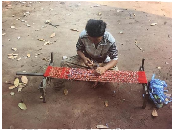
Figure 43 A woman tying matmi pattern into silk yarn, tensioned on a lakmee frame, Khon Kaen province.
