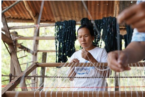
Figure 41 The weft threads are wound from a rack of bobbins onto a revolving frame, Thailand.
