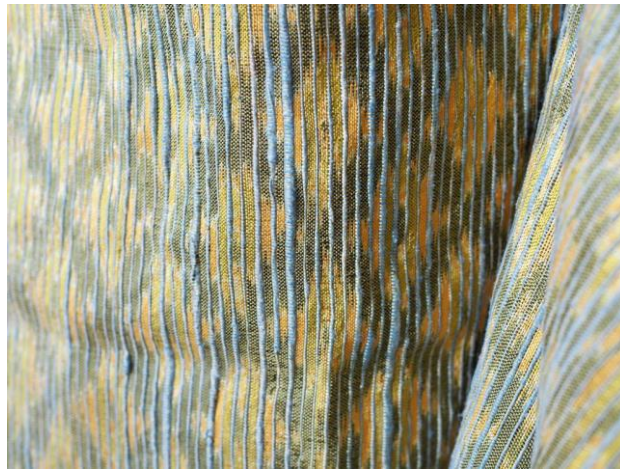
Figure 22 Woven fabric from Eri Silk. Weft Ikat patterns woven in plain weave.
