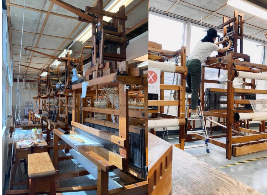
Figure 111 Tools and Equipment (Hand-dobby loom) to create weave structure
