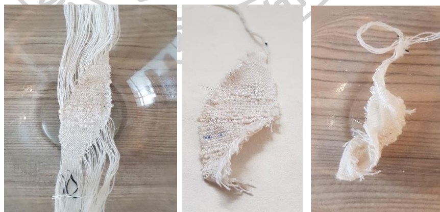
Figure 55. Left, before soak in hot water, middle, when cut warp yarns and the piece of experiment autonomy performed curved itself, and right after soak and twist.
