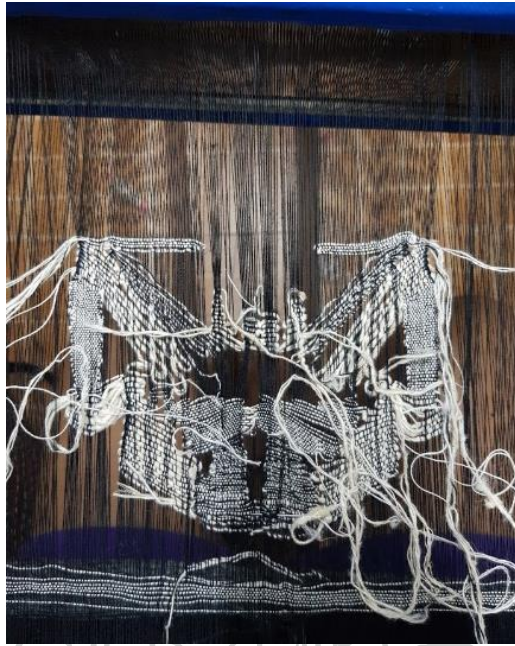
Figure 80. Simulate facial muscle by weave in irregular direction to examine the weft direction and the texture effect after wash.
