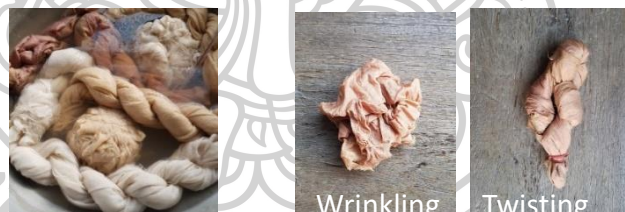
Figure 34. Boiling in hot water temperature about > 95 degree and dried without release twist formed.
