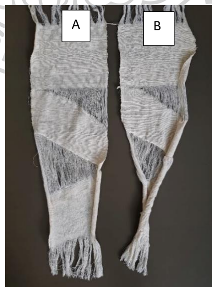
Figure 60. Experiment to compare the weft yarn of single weft and yarn twist weft.
