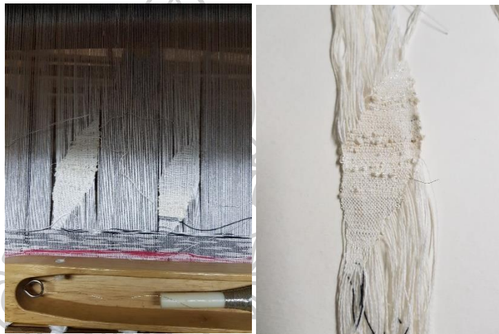
Figure 54. Left, twist yarn in shaped weaving on loom and right, when remove the piece of experiment from loom.
