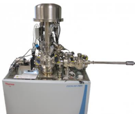
Figure 23: X-ray photoelectron spectroscopy (AMICUS photoelectron spectrometer)
