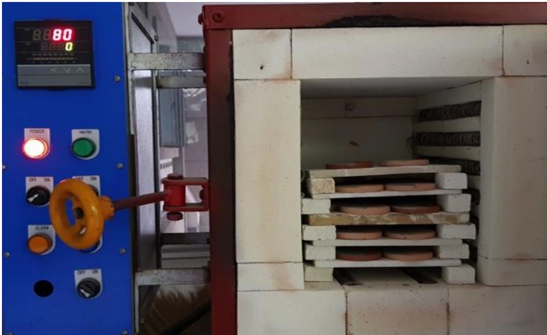
Figure 73 Put test pieces into the kiln for firing at 1,222 °c.
