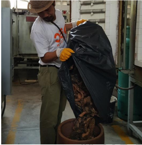
Figure 61 - 62 Put dried durian rinds into a pot for firing in the kiln at 800 °c.
