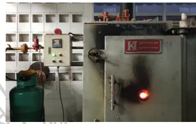
The Gas kiln can be use for glost firing in atmosphere reduction and oxidation. Photo by researcher.
