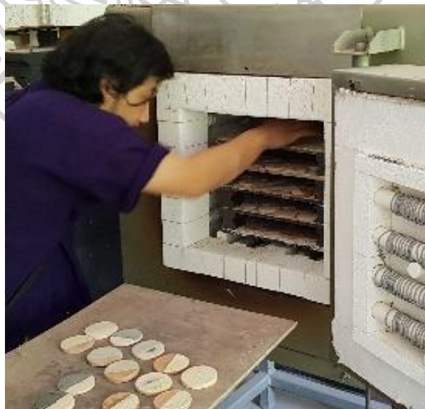
Figure 71 - 73 Painted glaze on earthenware and stoneware clay body test plates.
