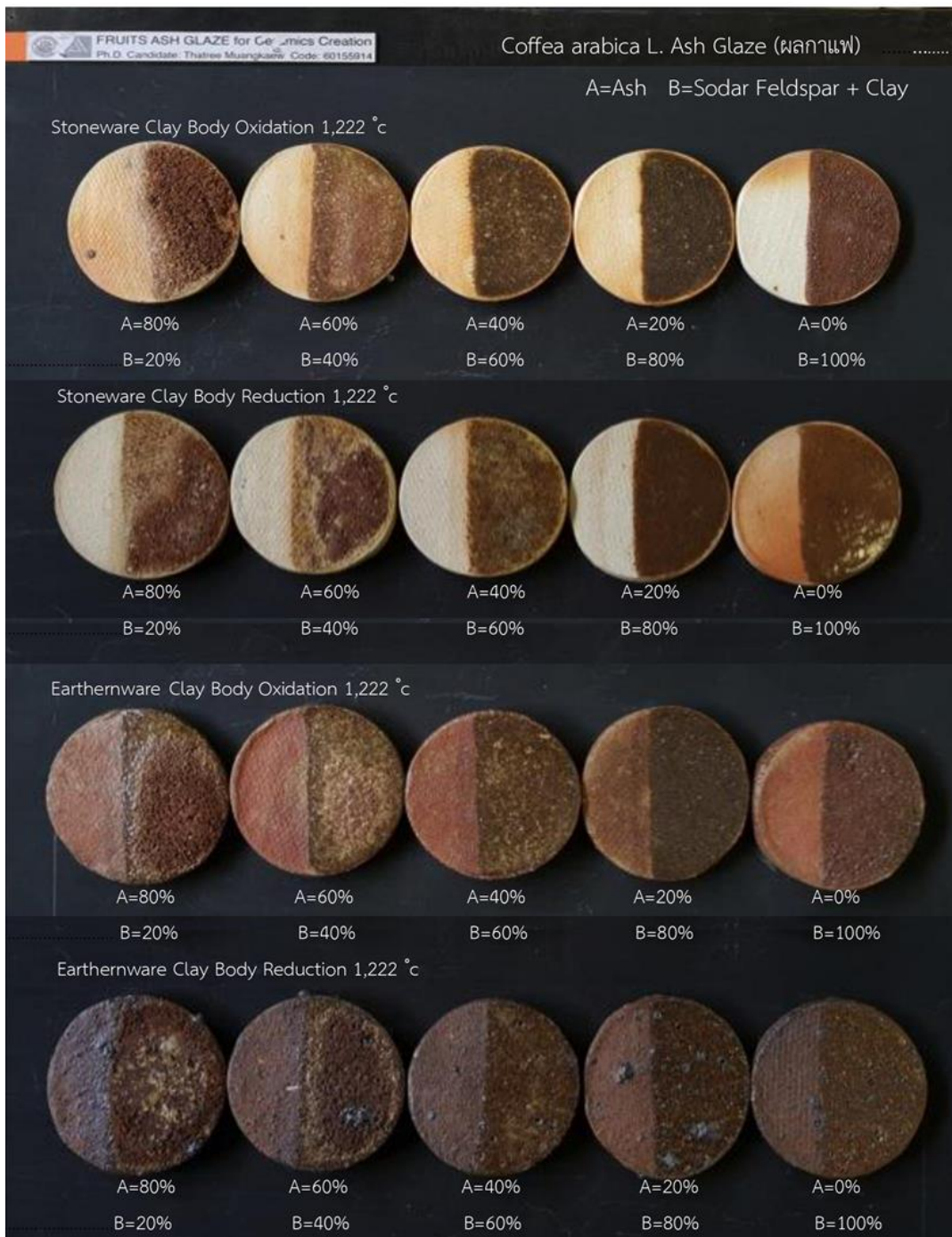
Figure 81 Coffea arabica L. Ash by Line blend glaze testing.
