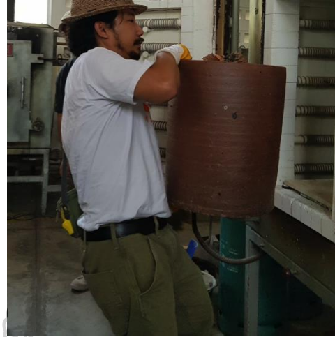
Figure 61 - 62 Put dried durian rinds into a pot for firing in the kiln at 800 °c.
