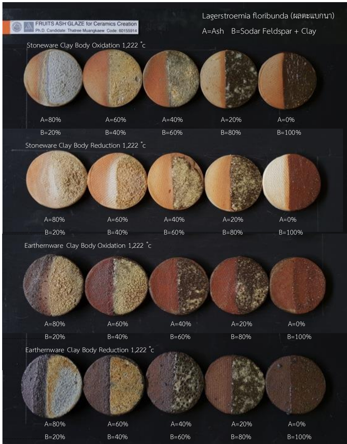
Figure 100 Line blend glaze testing with Lagerstroemia floribunda Ash, 2019.
