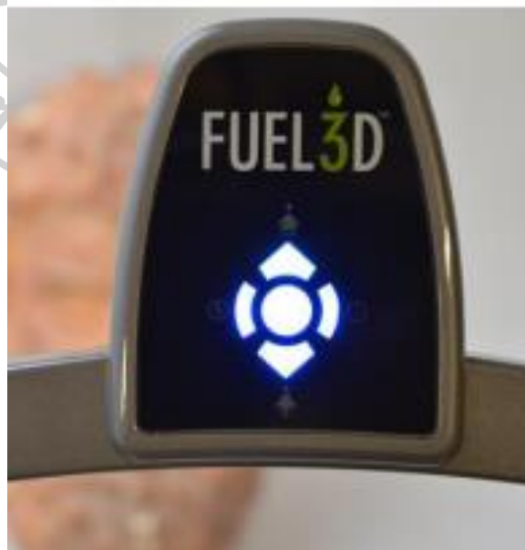
Figure 18 When the scanner reaches the correct range from the target then all LEDs will light up. All LEDs light up the scanner is ready to scan
