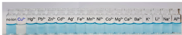
Fig. 7. Colors of the Cy7C4 sensor (10 \mu\text{M} ) before and after the addition of \text{Cu}^{2+} , \text{Hg}^{2+} , \text{Pb}^{2+} , \text{Zn}^{2+} , \text{Cd}^{2+} , \text{Ag}^+ , \text{Fe}^{2+} , \text{Mn}^{2+} , \text{Ni}^{2+} , \text{Co}^{2+} , \text{Mg}^{2+} , \text{Ca}^{2+} , \text{Ba}^{2+} , \text{K}^+ , \text{Li}^+ , \text{Na}^+ and \text{Al}^{3+} (5.0 \mu\text{M} ).
