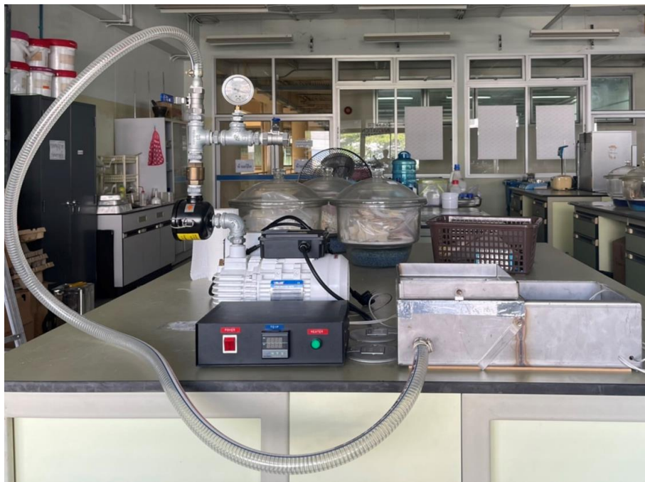
Figure 59 Thermoforming equipment in Polymer Innovation Laboratory.
