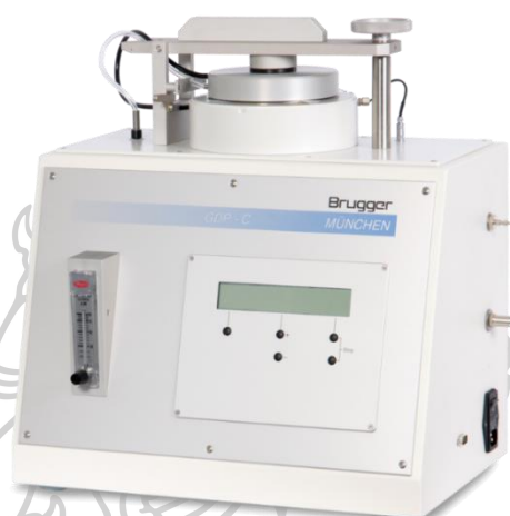
Figure 15 Gas permeability tester (Brugger Feinmechanik, Munich, Germany).
