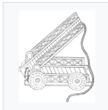
Mobile moat crossing bridge
