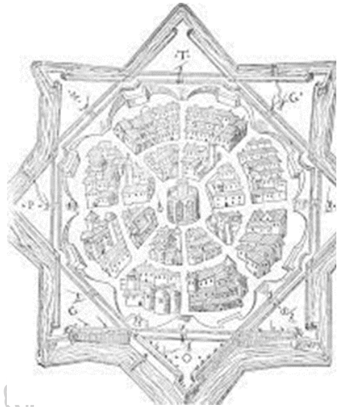
Figure 28. Plan of "Sforzinda" with radial avenues (Source: Alverino, 1464)
