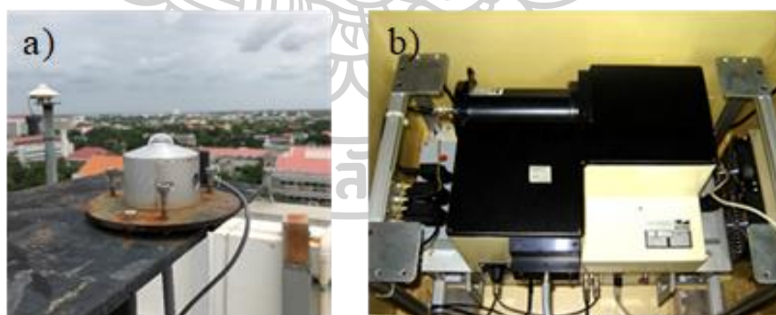
Figure 1 A pictorial view of the spectroradiometer installed at Nakhon Pathom a) input optics b) the monochromator and detector
