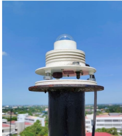
Figure 24 Broadband UV radiometer model 501A of Solar Light company at Nakhon Pathom station.
