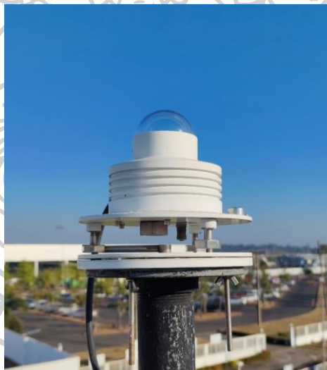
Figure 25 Broadband UV radiometer model 501A of Solar Light company at Ubon Ratchathani station.
