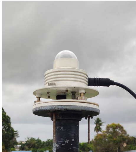
Figure 26 Broadband UV radiometer model 501A of Solar Light company at Songkhla station.
