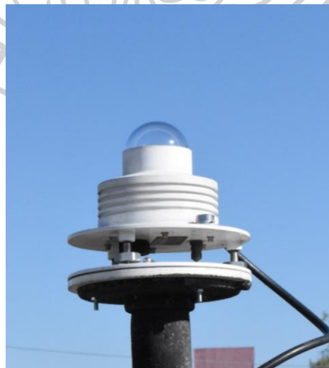
Figure 23 Broadband UV radiometer model 501A of Solar Light company at Chiang Mai station.
