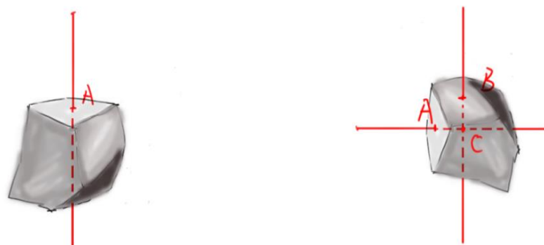
Figure 62A-B: The suspension method looks for the center of gravity of an irregular object
