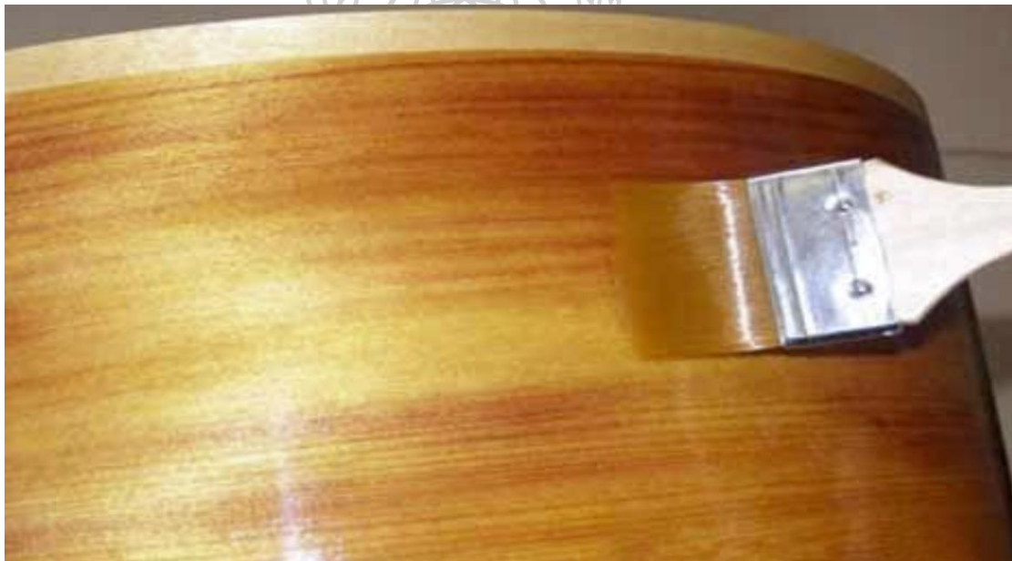
Figure 52 Step 8: Apply the wood paint
