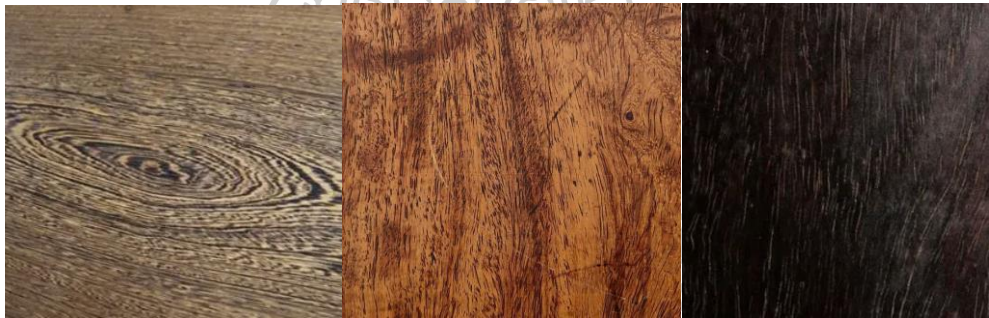
Figure 5 The characteristics of rosewood, chicken wings, and yellow rosewood pattern characteristics commonly used in Ming -style furniture
