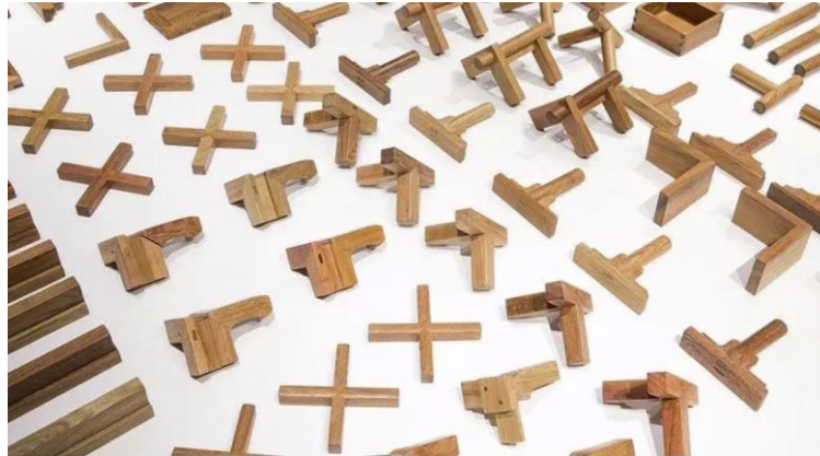
Figure 10 The diversity of Ming -style furniture tenon and tenon
