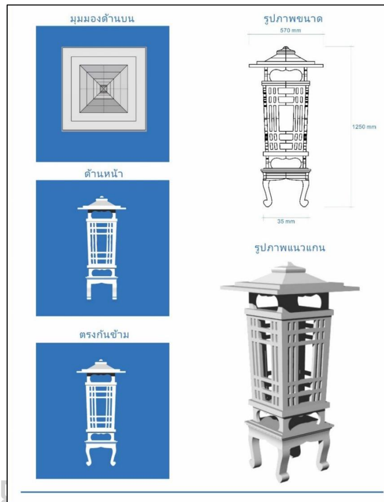
Figure 95 Prototype 1 of courtyard lamps (with roof elements)
