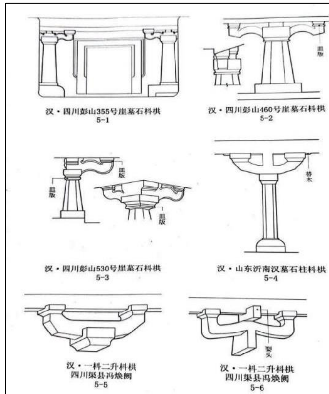
Figure 9 The arch structure of the Han Que, Note: Image quoted from Source: Mr. Liu Dunzhen, History of Ancient Chinese Architecture
