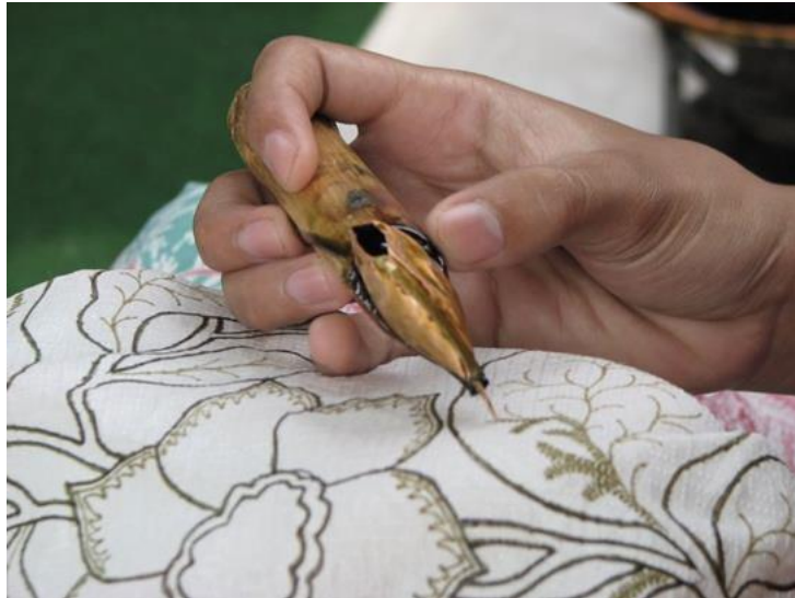
Figure 4 Hand drawing batik using a canting to apply wax-resist to cloth. (Retrieved November 20, 2020 from https://ich.unesco.org/en/RL/indonesian-batik-00170 )
