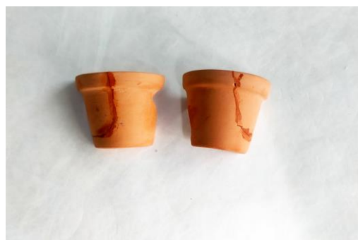
Figure 33: The residues from Altaco and X'traseal penetrate deep into the terracotta's structure.
