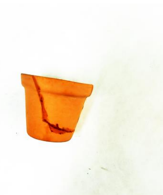
Figure 34: Risks of UHU glue on Terracotta sample.
