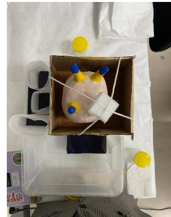
Figure 64. Applying gentle pressure on the glued parts using cotton strings.
