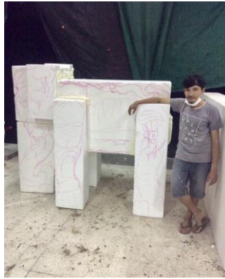
Figure 22. After cutting, combine the foam follow the shape, glueing each other foam parts by PU foam.
