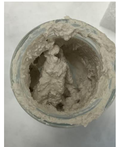
Figure 67. Mix between the marl powder and lime together.
