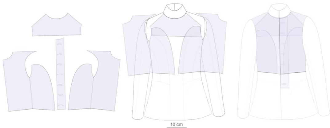
Fig. 72: Illustration of the cotton felt lining (purple colour).
