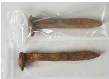
Fig. 139. Simple zip-lock bags for reducing corrosion risks caused by external sources of pollutants.
