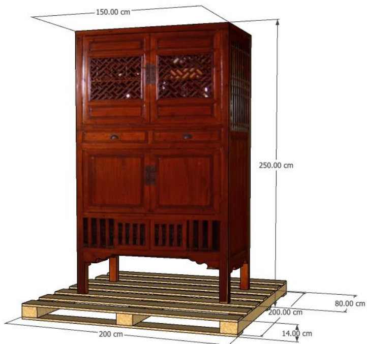
Fig. 181. The storage arrangement of wooden cabinet on pallet. Source: Miss.Pornganok Sadakorn (15 August 2023)
