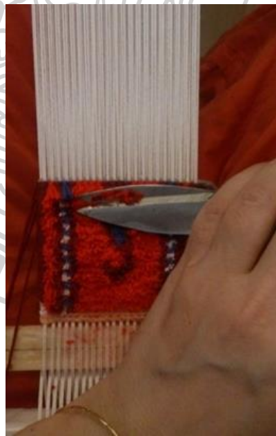
Figure 58 : Cutting the ends of the knots by scissors.
