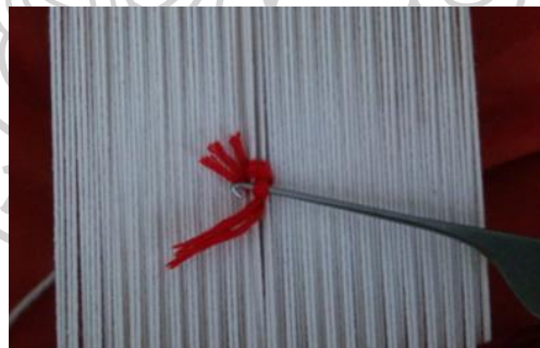
Figure 54 : Pulling out the head of the knot and completing the knot.
