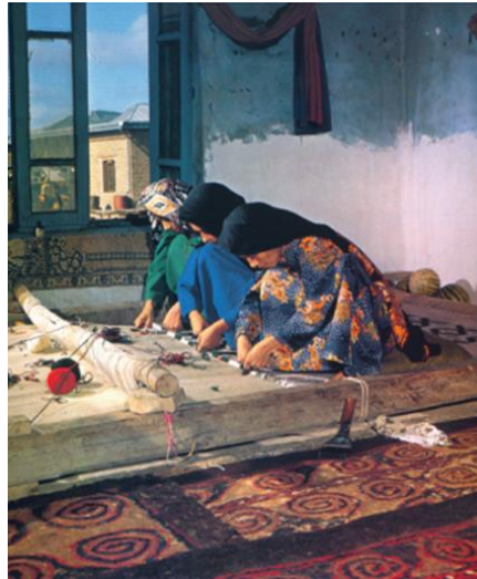
Figure 29 : The method of weaving on the horizontal loom.
