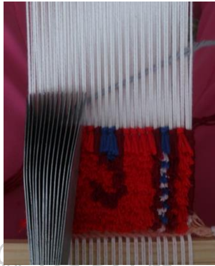
Figure 57 : Passing the weft thread over the knots.
