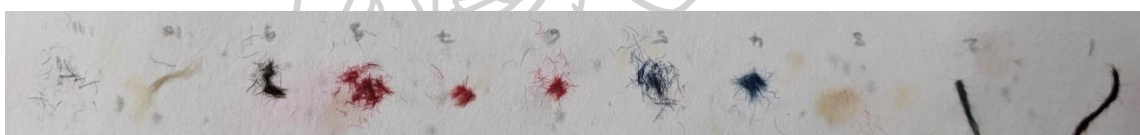
Figure 99 : Test on 11 samples isolated from knots and blue weft thread.
