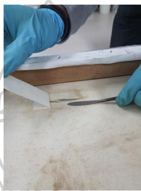
Figure 31: Removing sticky tape by pulling. 21 March 2023.
