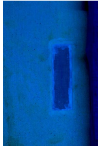
Figure 18: Excess adhesive around the sticky tape visible in UV light. 15 March 2023.
