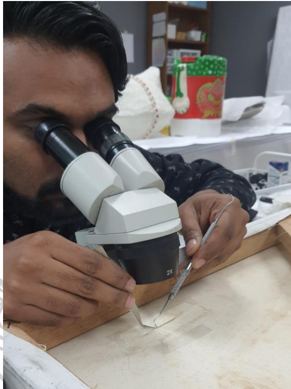
Figure 33: Tear mending under stereo microscope. 3 April 2023.
