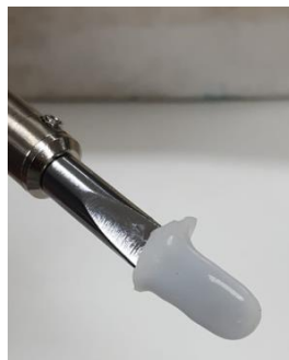
Figure 28: Spatula after silicon coating is completely dry. 2 February 2023.
