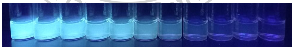
Figure 10 CDs solution with adding of \text{Hg}^{2+} at various concentrations under the UV light
