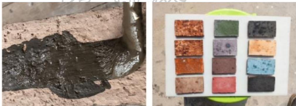
Figure 155. Colored clay slip test
