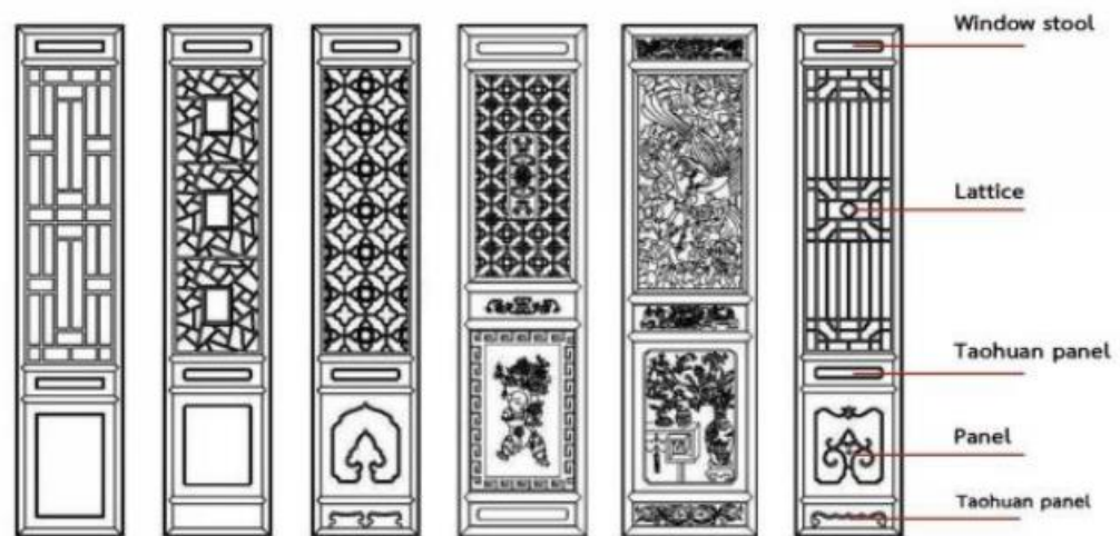
Figure 10. Long window structure
