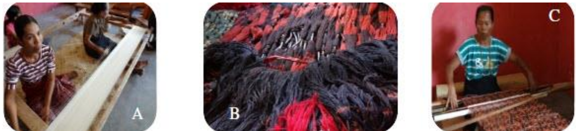
Figure 7. Production Woven Fabric, A. Pamering B. Yarn that has been tied and dyed, C. Weaving activities
