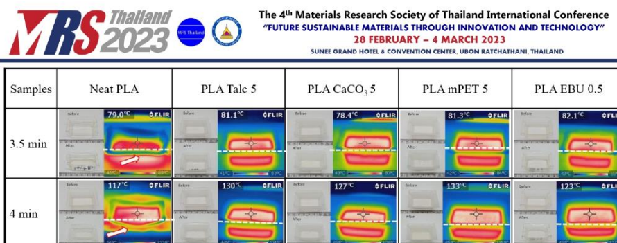
Figure. 5 Microwave heating of PLA Talc, PLA CaCO 3 , PLA mPET and PLA EBU trays filled with olive oil tested in the microwave heating power 600 W for 3.5 and 4 min.
