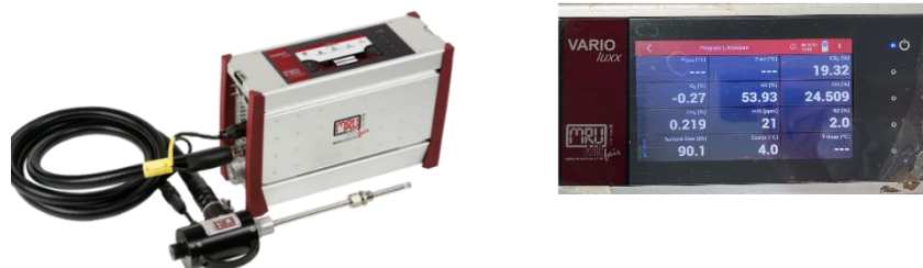
Figure 22. A gas analyzer (GA), MRU model, Vario luxx
