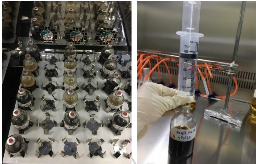
Figure 15. Biohydrogen production in serum bottles and gas measured by a syringe
