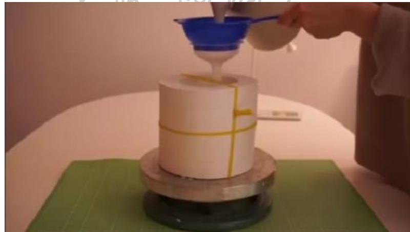
Figure 17 Slip casting technology
