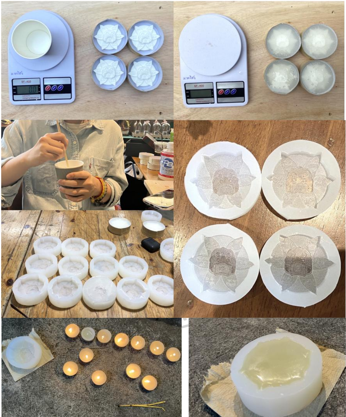
Figure 25: Silicone Mold Turnover process
