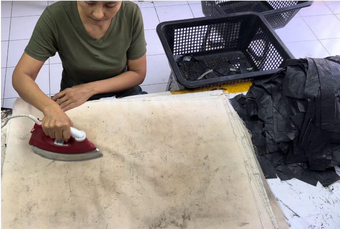
Figure 83 Smoothing out the leather by ironing before proceeding to the next step
