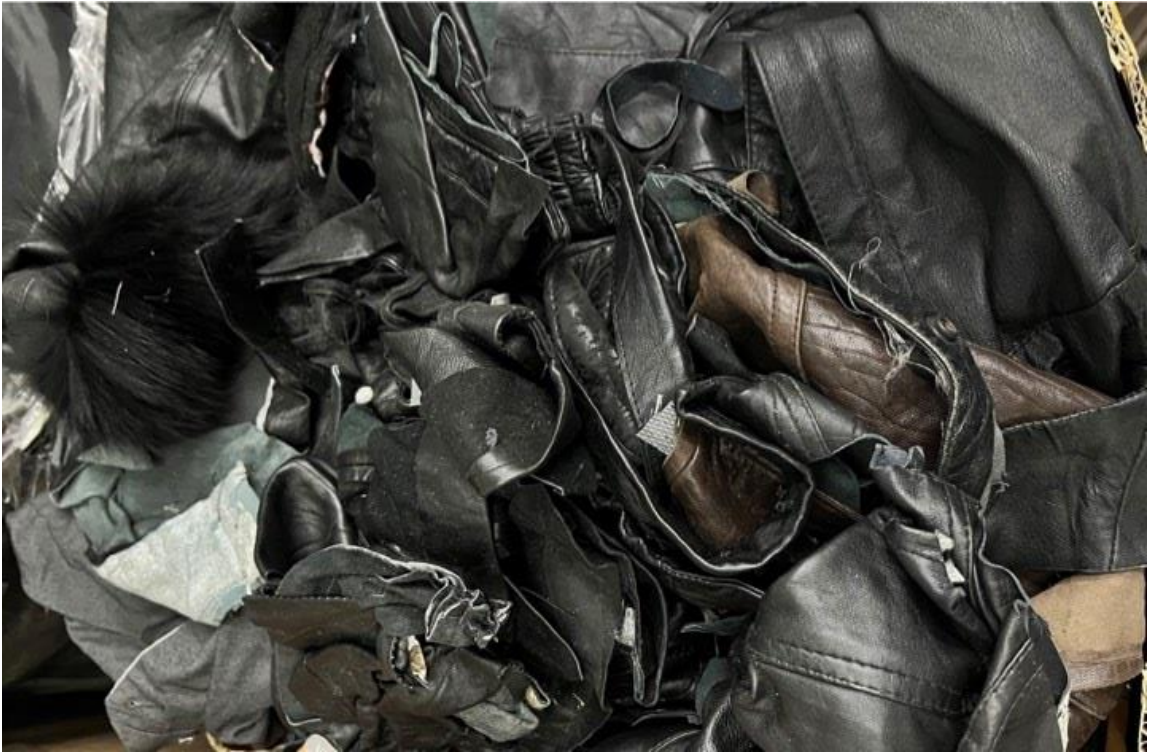
Figure 4 30-40% of the leather left over from cutting and sewing becomes scraps that are difficult to recycle.
