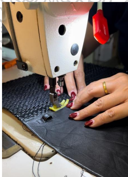
Figure 79 Loom woven leather sheet is sewn together to leather from a jacket.
