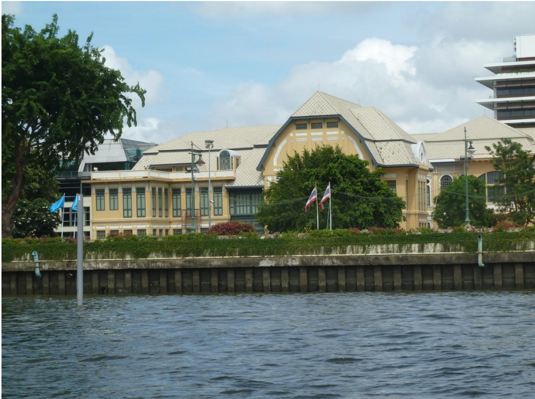
Figure 22 Rama VI ‘domestic’ style in masonry and translated to a large institutional building: again there are complex roof forms, hybrid hip-and-gable, dormers in various forms.
