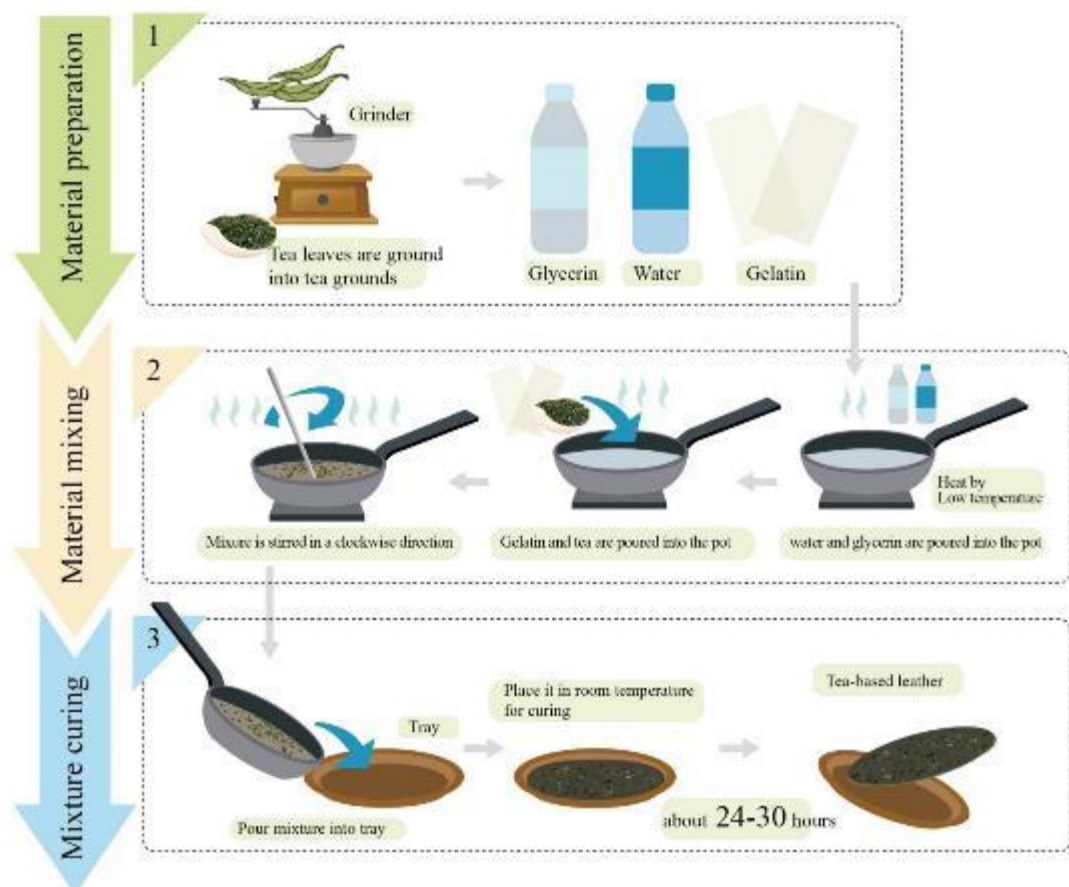
Figure 30: The process of material experiment with glycerin and gelatin
