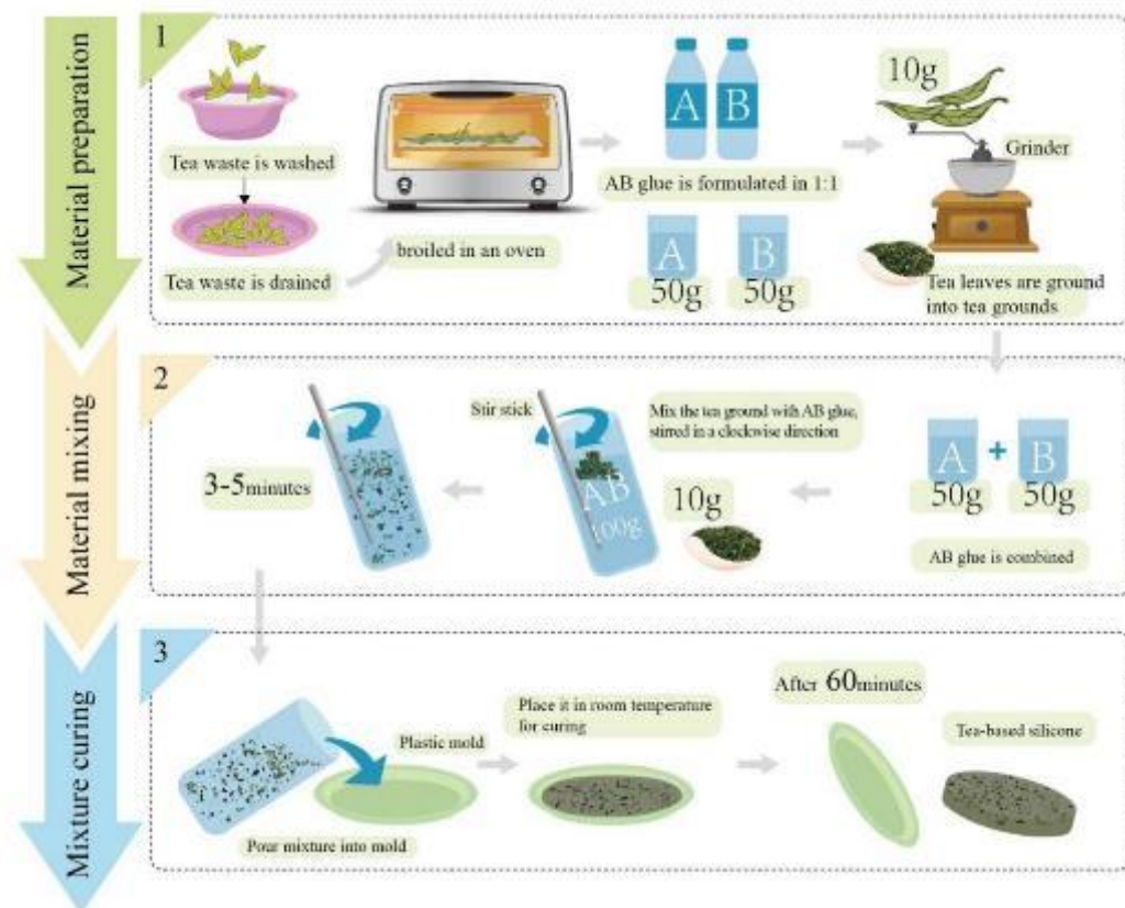
Figure 26: The process of material experiment with Silica Gel
