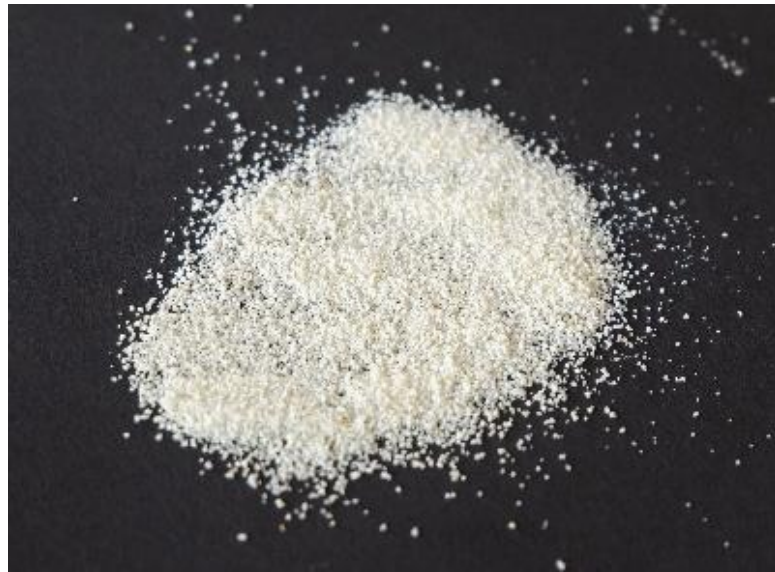
Figure 3.5 MMA-g-LNR powder image obtained from graft copolymerization using as compatibilizers for PLA/PP blend.
