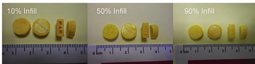
Figure 12. Images of tablet which have different percentage infill (from left to right): top, base, internal and lateral views.
