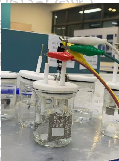
Fig. 3.7 Photograph showing the geometric arrangement of the Ni foam working electrode and zinc counter electrode in the electrolyte
