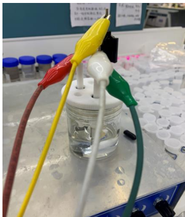
Fig. 3.6 Photograph of the experimental setup for electrodepositing Zn/Ni foam composite anodes
