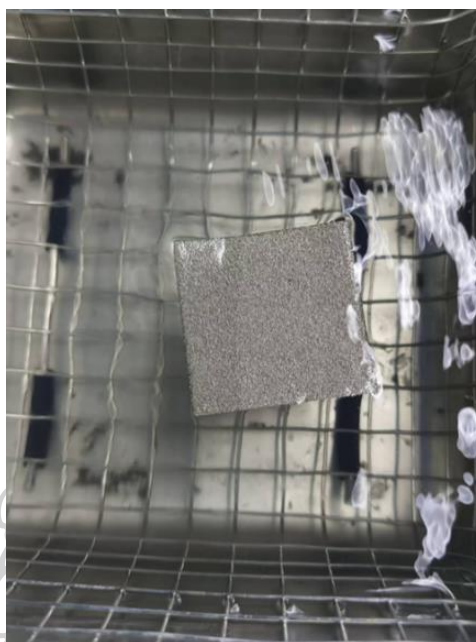
Fig. 3.4 Photograph of Ni foam undergoing ultrasonic acid pickling in an HCl/water mixed solution
