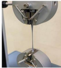
Figure 3 Elastic materials tests using a universal tensile testing machine
