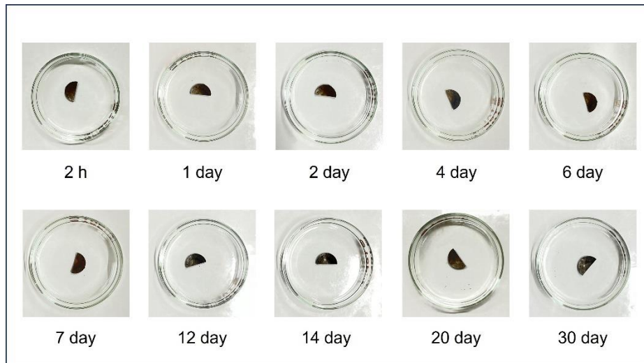
Figure 17 Stability in water of the cerium-modified Im_GO membrane for 30 days.
