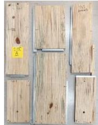
Figure 55 : Close-up of interlocking jigsaw design using grooves.
