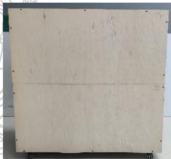
Figure 53 : Closed box using foldable plywood and iron nails.
