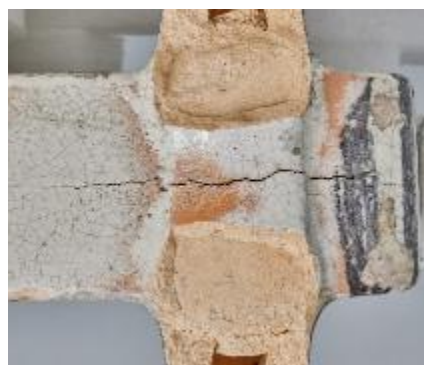
Figure 24 : Close-up of a major crack due to impact damage.
