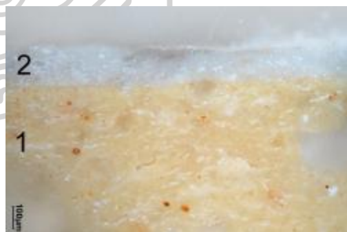
Figure 15 : Micrograph of clay body cross-section.
