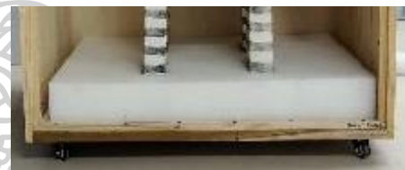
Figure 56 : Close-up of Ethafoam custom-cut to fit legs of Textured Dog.
