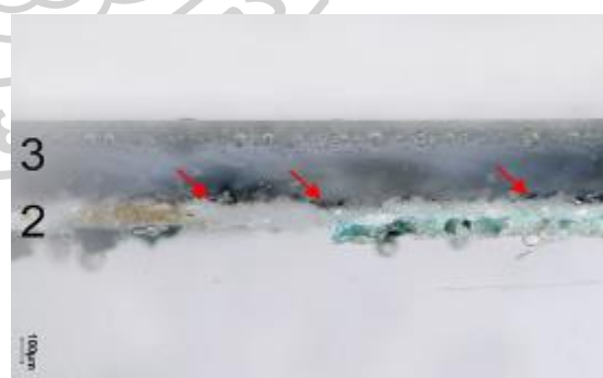
Figure 19 : SEM-EDS showing black glaze pigment (red arrow) and green biological growth.
