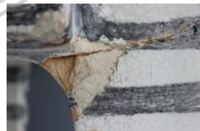
Figure 27 : Close-up of area where clay body has been lost due to impact damage.
