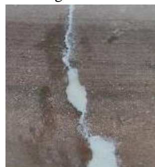
Figure 35 : Close-up of Epo filling on mock ceramic pot.
