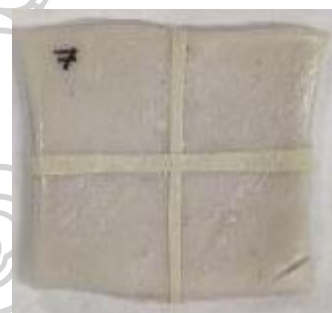
Figure 37 : Epo putty square for protective coating testing.
