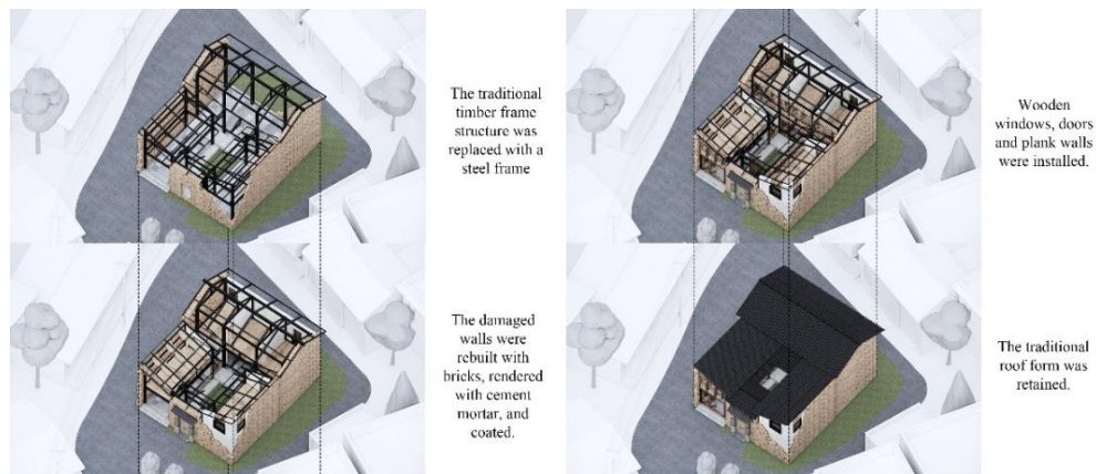
Figure 99 Messing Analysis and Structure
