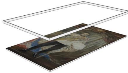
Figure 20: Drawing of inner frame in conjunction with strainer.
