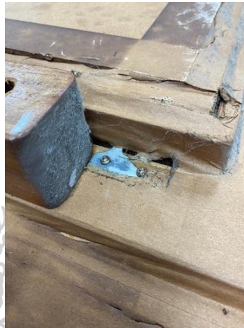
Figure 81: Tool covered with paper tape, holding frame and auxiliary support together.
