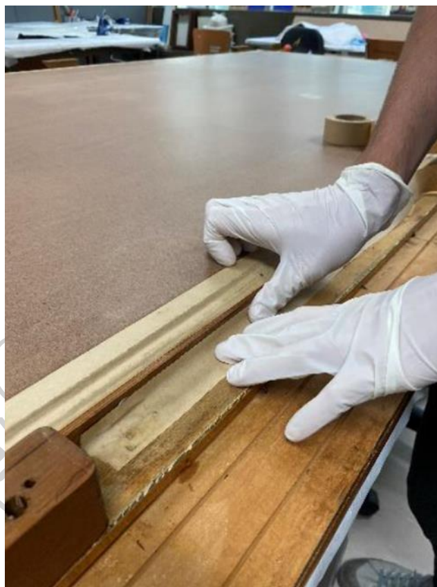
Figure 125: The water-activated paper tape was added to finish the framing.
