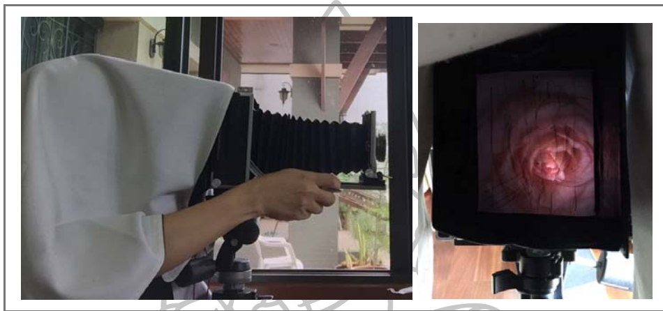
Figure 59 Dark cloth helps getting rid of distracting ambient light while focusing. The image appears upside down on the ground glass
