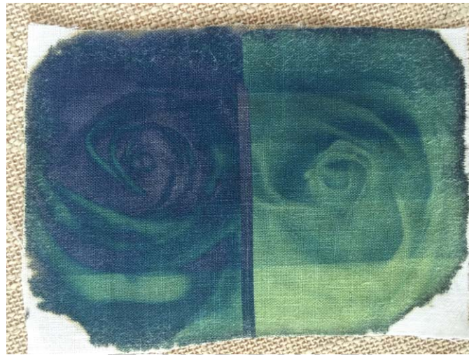
Figure 68 Test strip is done with the increment of 5 minutes each.
