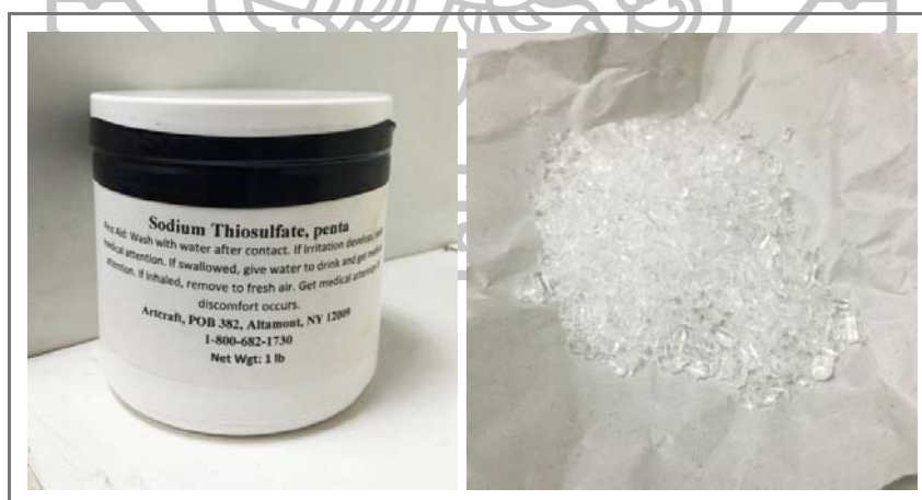
Figure 73 Sodium Thiosulfate appears clear crystalline
